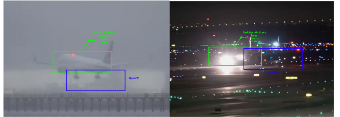
Figure 6. Shots of the final output performing on the two real-world dynamic examples. As shown, the implementation correctly tracks both aircraft, and performs better than Open CV's mean point approach depicted in blue
